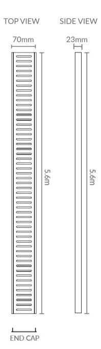
\* Total length of full grate is 5.8m, total usable length is 5.6m to allow for any wastage during the anodising process.
